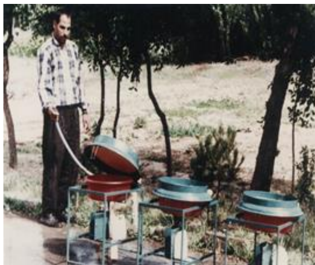
Figure 2. Automatic rain sampler used for collecting precipitation samples at various elevations.
