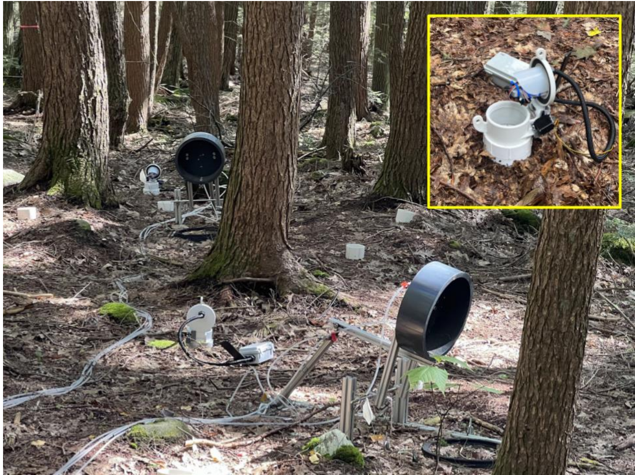
Photo 1 | Field deployment of soil CO 2 flux monitoring systems at Harvard Forest. The image shows both Fluxbot 2.0 and autochamber systems deployed side-by-side in a hemlock forest stand. The larger pneumatically-operated autochambers are connected via tubing to a central control box containing the infrared gas analyzer (IRGA), while the smaller autonomous Fluxbot 2.0 units operate independently with integrated CO 2 sensors and servo-actuated lids. The inset shows a close-up of a Fluxbot 2.0 unit with its hinged lid design and compact, battery-powered configuration. This co-located deployment enabled direct comparison of flux measurements between the two systems under identical field conditions.
